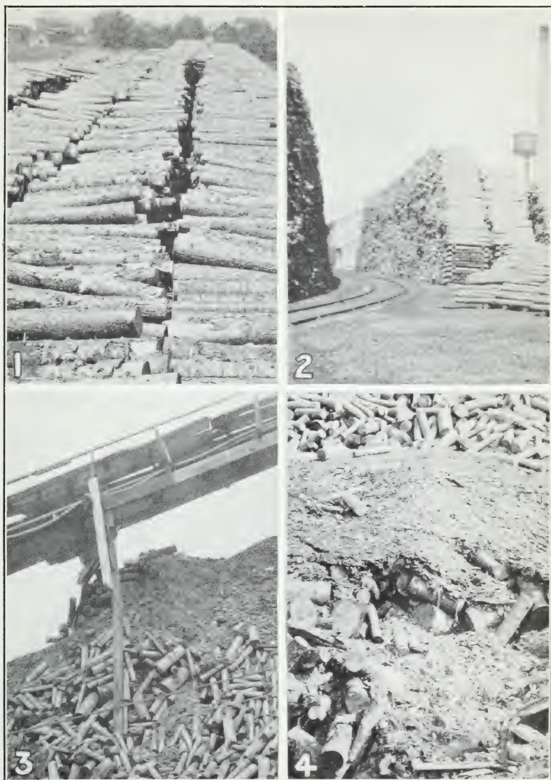
FIG. 1.—Ranked piles of 8-foot spruce. This type of piling, without adequate ventilation at the sides and beneath the ranks, leads to serious decay in a comparatively short time
